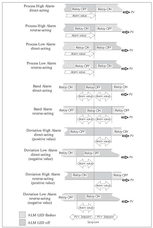
Figure 2-2 Alarm Operation
